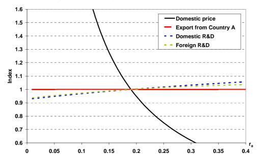
From Proposition 3 above we know that the price of the technology falls when the standard increases. In Figure 1 we see that this price effect is very significant. The price is approximately halved when the emission standard is doubled.
